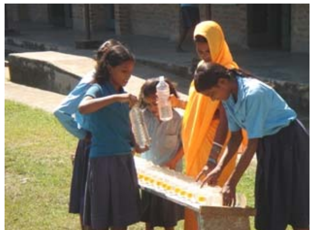
School club members put SODIS bottles out for treatment. The stand holds 25 bottles and is tilted on one side for proper sun exposure. (Photo: A. Shrestha)
